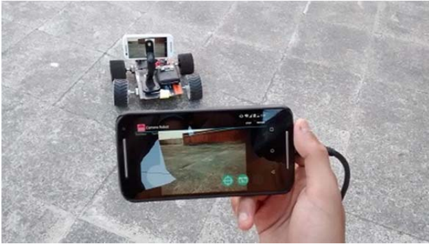
Fig. 11 Video captured by the phone mounted on the robot is being displayed in the Application in the Controller Phone.
