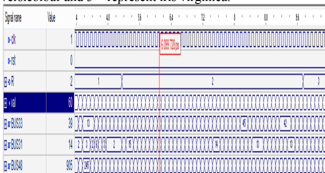
Fig.5 simulation results for hardware implementation of neural network ( iris data sets)
