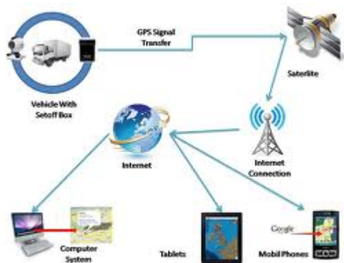
Fig. 5 How GPS Tracking System works
